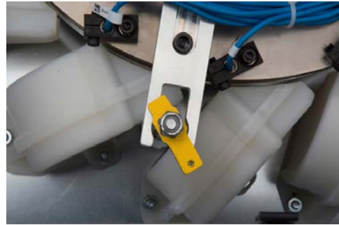
Incorrect: disk is not secured
