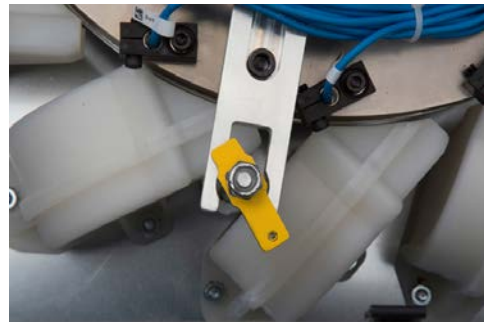
Incorrect: disk is not secured
